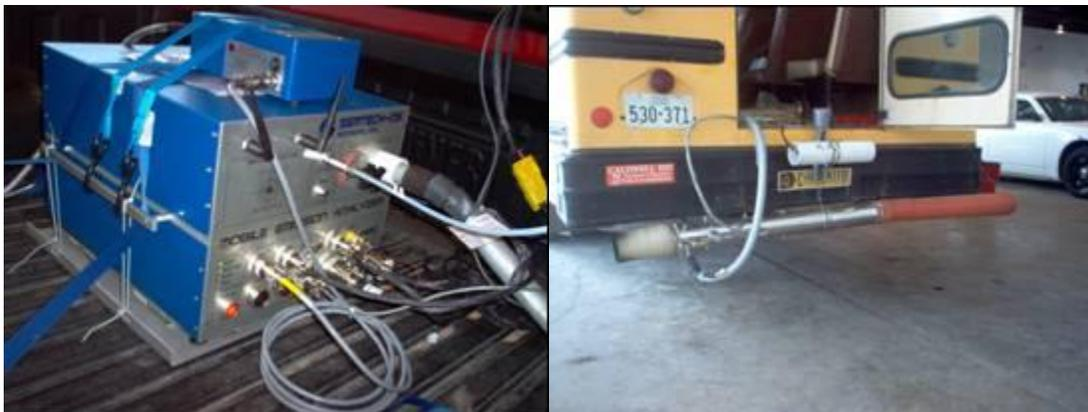
**Figure 4. Components of the SEMTECH-DS Unit Installed on a School Bus.**
