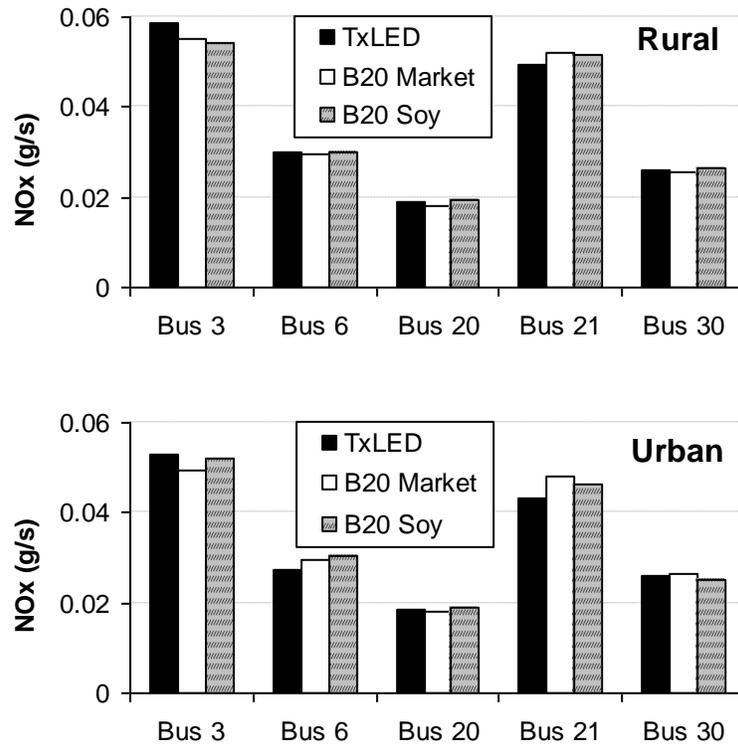
**Figure B6. Individual Bus Average NOx Idling Emissions Rates.**
