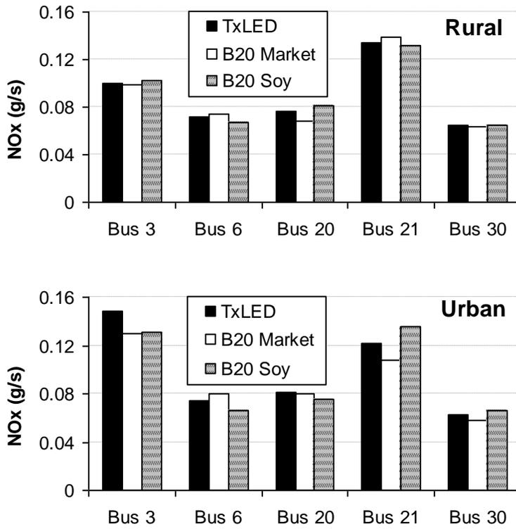
**Figure B8. Individual Bus Average NOx Emissions Rates for Cruising at 40 mph.**
