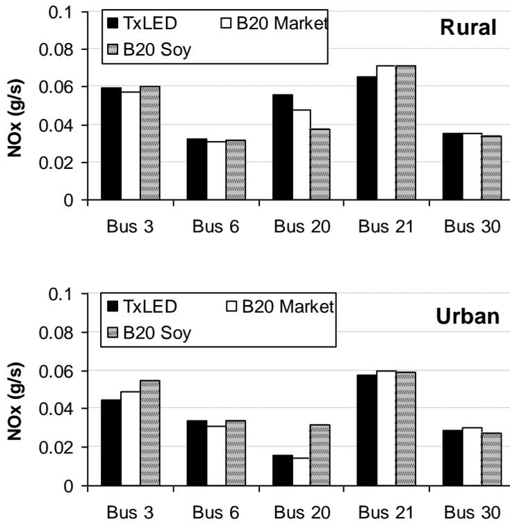
**Figure B7. Individual Bus Average NOx Emissions Rates for Cruising at 20 mph.**
