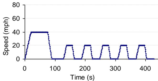
**Figure 3. Synthetic Driving Cycle Representing Urban Driving Conditions.**
