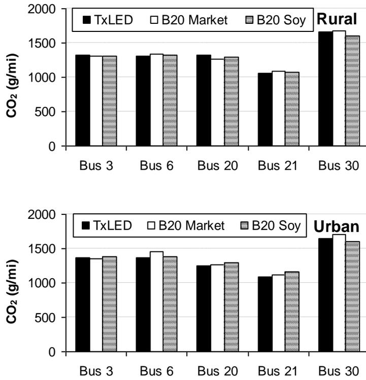
**Figure B3. Average Individual Bus Mass CO<sub>2</sub> Emissions Rates.**
