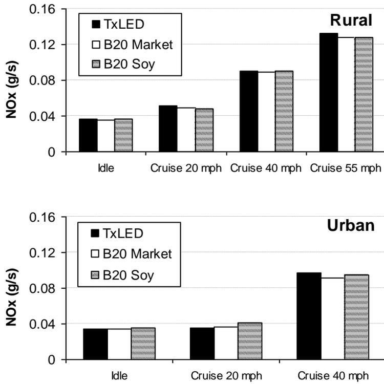
**Figure B5. Average Texas Fleet NO<sub>x</sub> Emissions Rates for Different Stable Speeds.**
