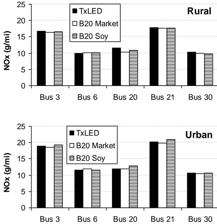
Figure B1. Average Individual Bus Mass NOx Emissions Rates.
