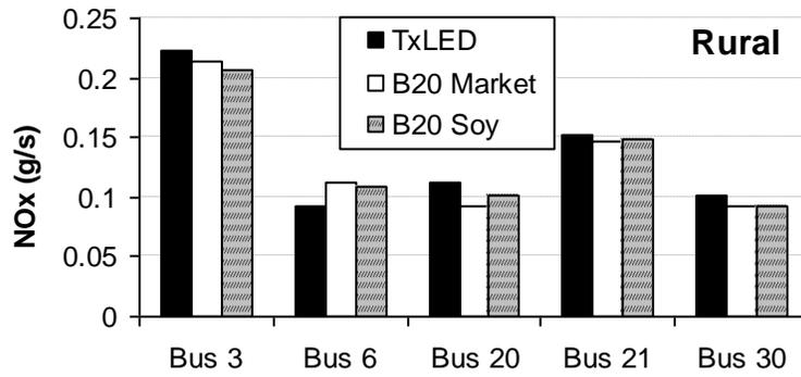
**Figure B9. Individual Bus Average NOx Emissions Rates for Cruising at 55 mph.**
