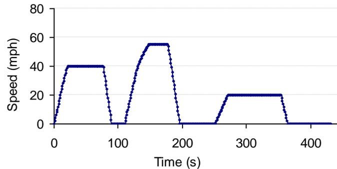
**Figure 2. Synthetic Driving Cycle Representing Rural Driving Conditions.**
